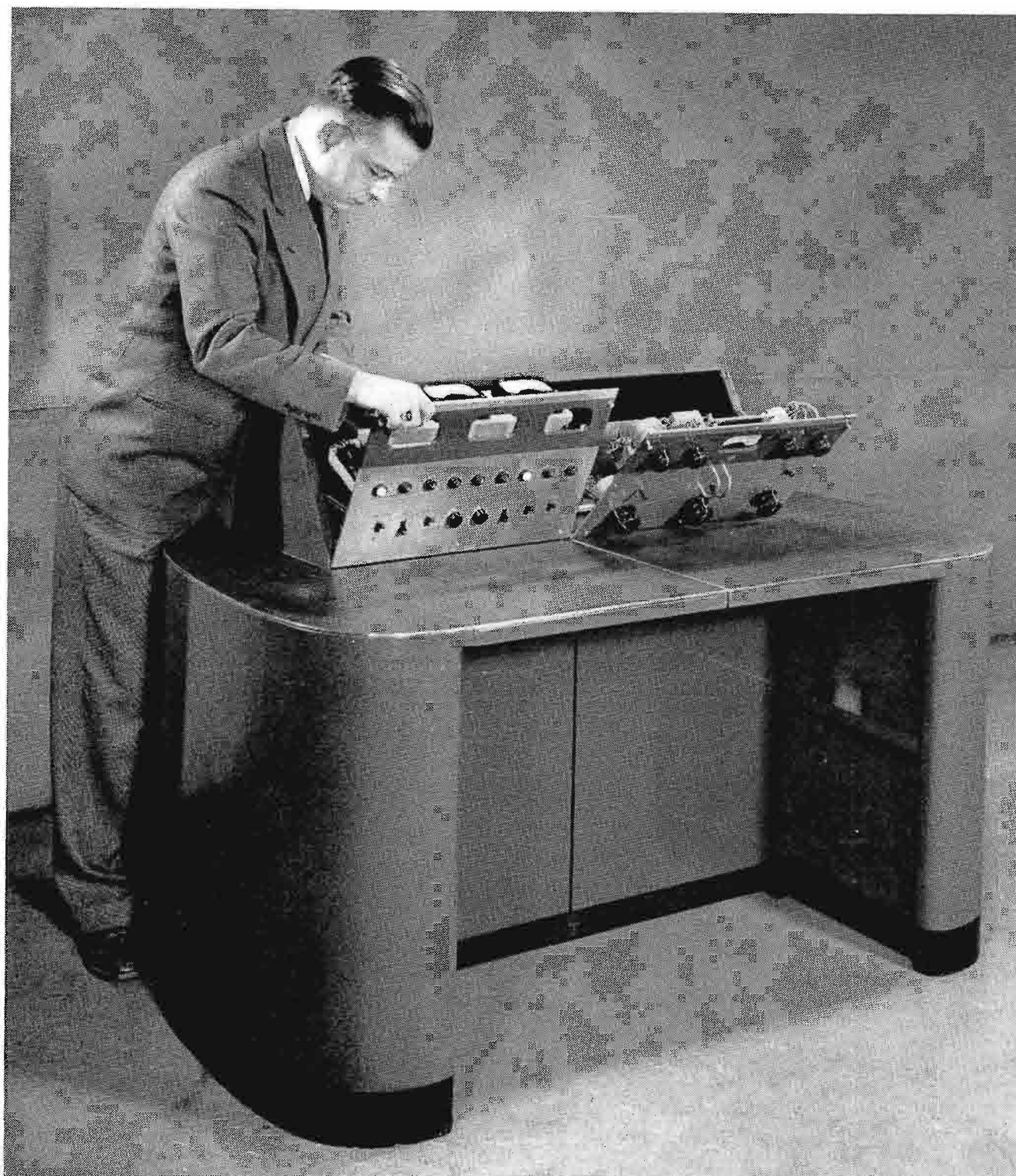
FIG. 14 (below). D. G. Robertson, RCA engineer, illustrates how hinged turret panels of the BTC-1A supervisory console provide complete accessibility. Note that individual meter panel may be tilted back for easy zero adjustments. Transmitter control turret is at left; audio control turret, at right.
